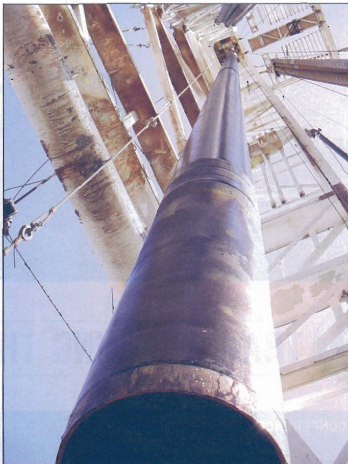
After expansion, the monobore liner extension system is pulled from the test well (Fig. 3).
